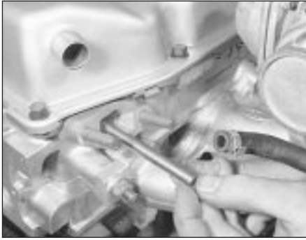
5.9 Removing the fuel pump push-rod
