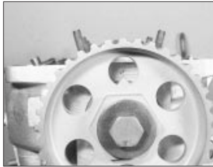
4.10b . . . and camshaft sprocket timing mark aligned with TDC mark on cylinder head
