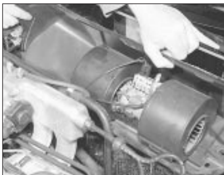
16.5b Removing the heater fan motor assembly . . .
