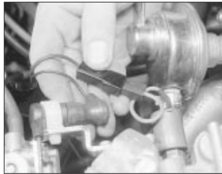
7.10b . . . anti-run-on valve and back bleed solenoid (if fitted) - 1.4 litre carburettor engine
