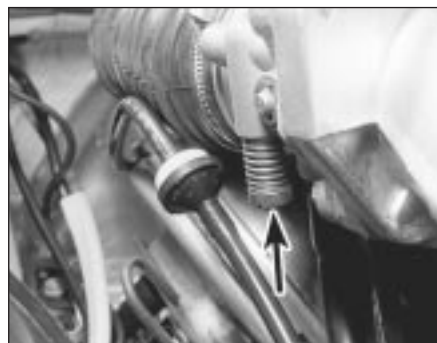
10.15 Idle speed adjustment screw (arrowed) on early K-Jetronic systems
