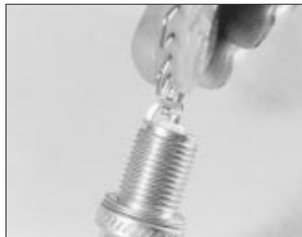
15.10b . . . and adjusting the gap using a special adjusting tool
