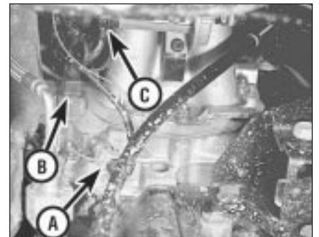
11.76 Coolant temperature sensor (A) thermo-time switch (B) and auxiliary air device (C) multi-plugs on RS Turbo models
