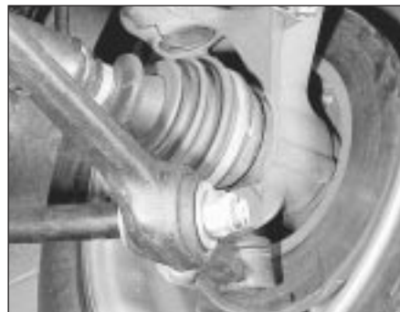
5.4 Anti-roll to lower arm retaining nut
