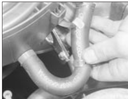
2.2 Disconnecting the crankcase ventilation hose at the air cleaner body
