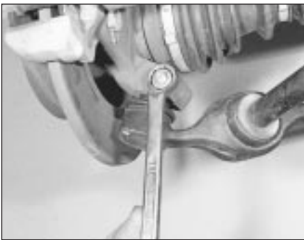
3.4a Removing the lower arm balljoint pinch-bolt nut
