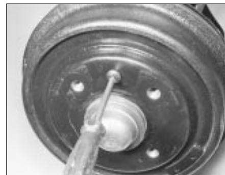
5.30 Removing the drum retaining screw on models with a separate brake drum
