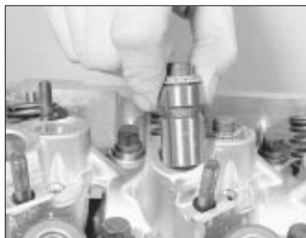
13.42 Fitting a cam follower to its bore
