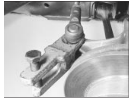
20.6 Releasing tie-rod balljoint using separator tool
