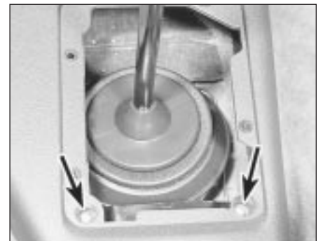
30.3a Centre console lower retaining screws (arrowed)
