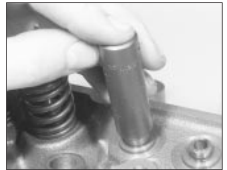
14.14d Using a long reach socket to push the seal fully home - HCS engine
