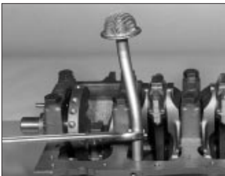
15.43a Line up the flange using a spanner - HCS engine
