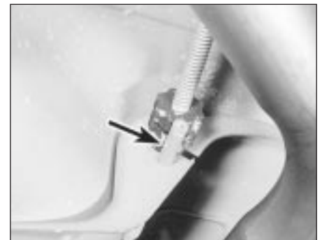
8.14 Handbrake cable adjuster nylon locking pin (arrowed)
