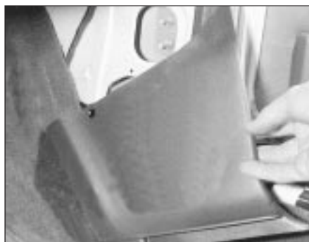
32.8 Removing cowl side trim panel
