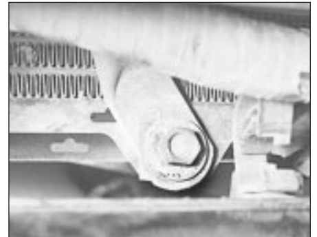
2.20b . . . to gain access to the fan shroud bolts on 1986 RS Turbo models
