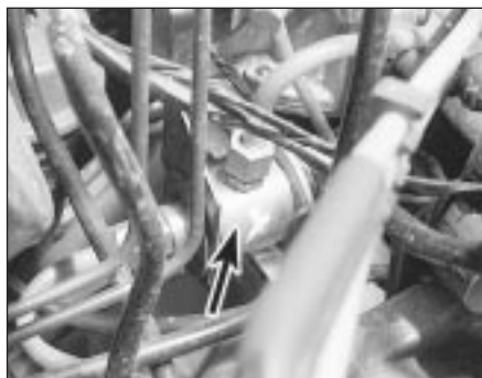
13.1 KE-Jetronic fuel pressure regulator location (arrowed) behind fuel distributor
