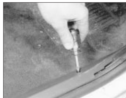
32.7 Removing a sill scuff plate securing screw
