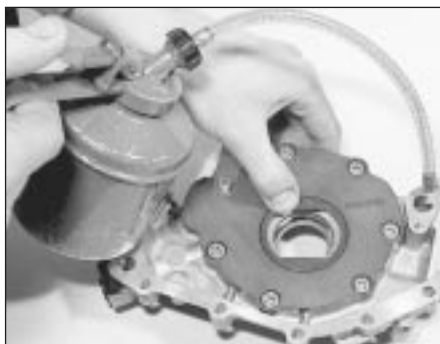
15.12 Priming the oil pump prior to fitting
