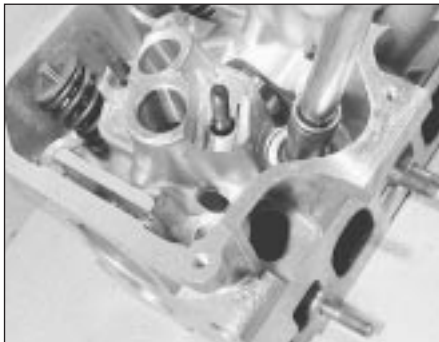
13.35 Using a socket to install a valve stem oil seal
