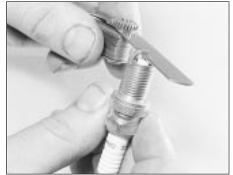
15.9 Measuring the spark plug gap with a feeler blade
