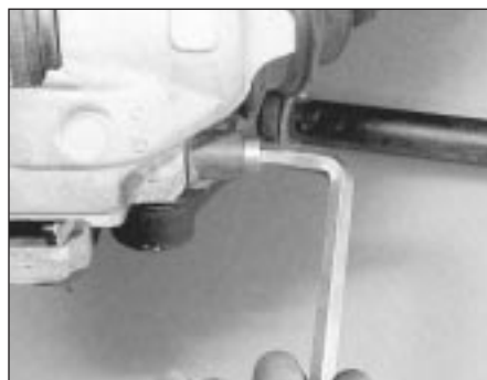
2.4a Unscrew the caliper bolt using an Allen key . . .
