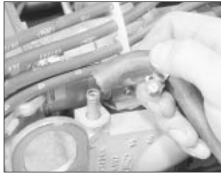
4.10 Disconnect the expansion tank hose at the thermostat housing - CVH engine
