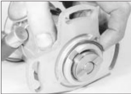
5.42 Checking the distributor O-ring seal condition - CVH engines (electronic breakerless system)
