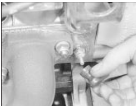
7.10a Disconnect the lead at the temperature sender . . .
