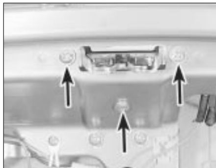
16.3 Tailgate lock retaining screws (arrowed)
