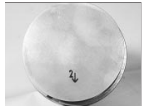
8.13b Arrow on piston crown must face the timing cover when installed
