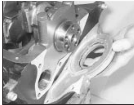
15.17 Fitting the crankshaft rear oil seal retainer
