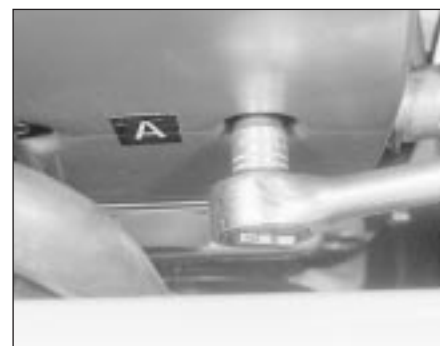
4.4a Where a two-piece timing belt cover is fitted, undo the bolts . . .
