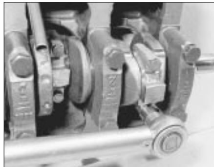
9.16b Tightening the big-end cap bolts to the specified torque
