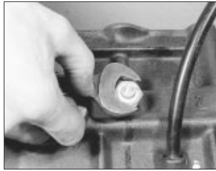
12.25 Unscrew the oil pressure switch
