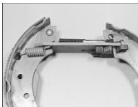
5.33a Brake shoe return spring and adjuster strut arrangement on Van, fuel-injected models and later Saloon and Estate models
