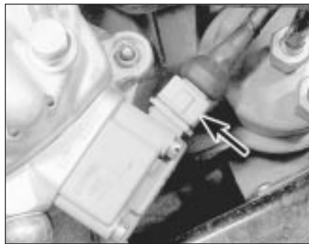
15.5 Pressure actuator wiring multi-plug (arrowed)
