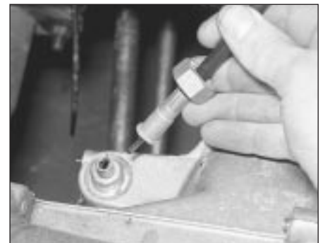
11.50 Disconnecting the speedometer cable - HCS engine
