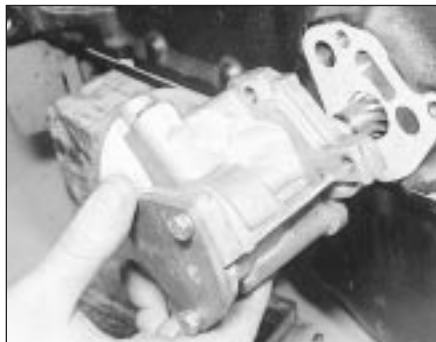
10.3 Removing the oil pump
