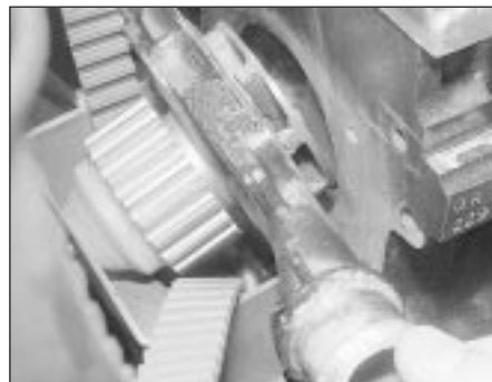
5.21b . . . and remove the water pump - CVH engine
