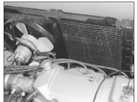
3.5b . . . and lift out the unit complete with fan - pre-1986 models (except RS Turbo)
