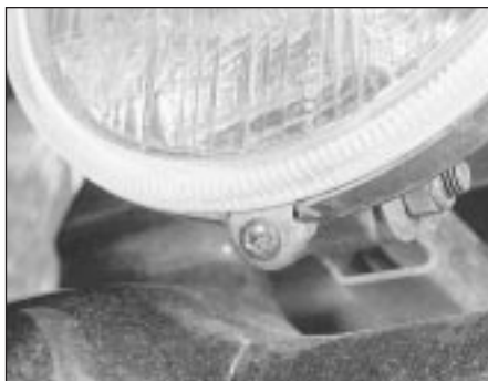
5.16 Front auxiliary lamp lens retaining screw
