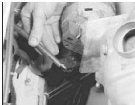
11.12a Disconnecting the alternator multi-plug . . .
