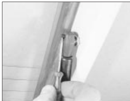
15.5 Releasing tailgate strut retaining clip
