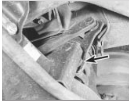
13.3 Anti-roll bar-to-lower arm shackle attachment (arrowed)
