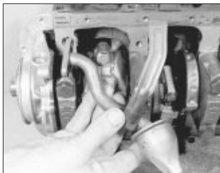
15.15 Fitting the oil pump pick-up tube
