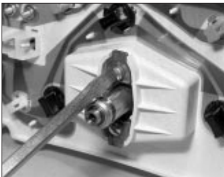
10.12a Extracting speedometer retaining screws
