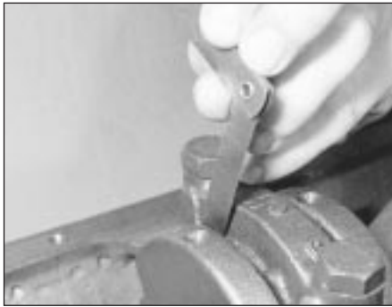
15.9 Using feeler blades to check crankshaft endfloat
