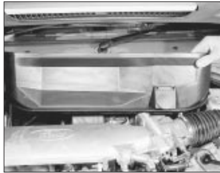
16.2 Heater plenum chamber removal
