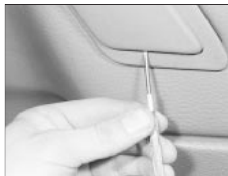
11.9a Prise out the door pull handle capping . . .
