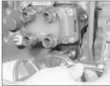
4.17 Removing a DIS coil securing screw - 1.3 litre HCS engine
