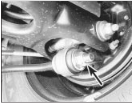
12.4 Tie-bar-to-stub axle carrier retaining nut (arrowed) - Saloon and Estate models
