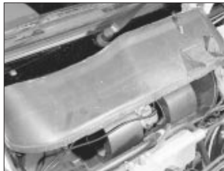
6.10b . . . and remove the plenum chamber top cover
