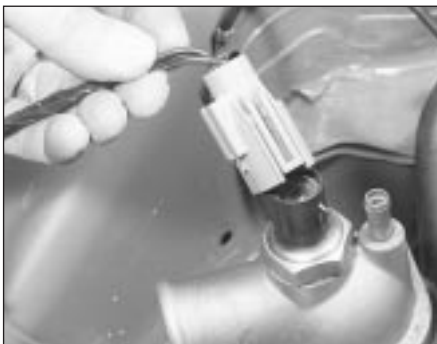
11.49a Disconnecting the cooling fan thermal switch . . .
