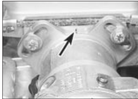
5.45a Distributor mounting flange and cylinder head punch marks (arrowed) - CVH engines (electronic breakerless system - early type distributor shown)
