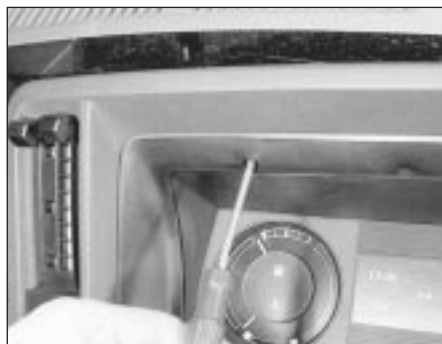
9.2a Extracting the instrument panel bezel screws - pre-1986 model
