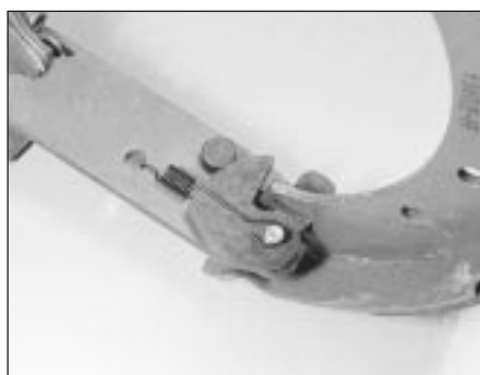
5.33b Automatic adjuster assembly on Van, fuel-injected models and later Saloon and Estate models
