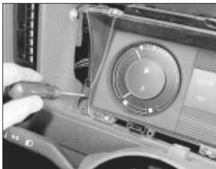
9.3 Removing an instrument panel retaining screw - pre-1986 model
