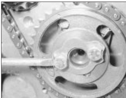
15.13 Secure the camshaft sprocket bolts with the locktabs
