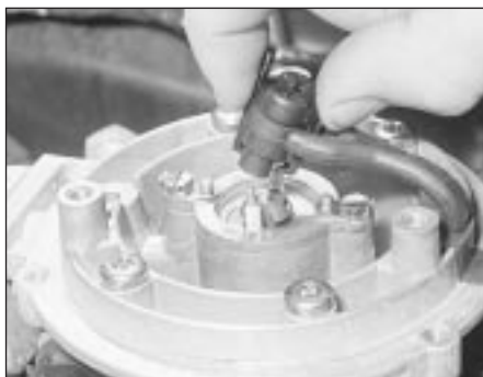
10.4 Disconnecting the fuel injector wiring plug - 1.4 CFI engine
