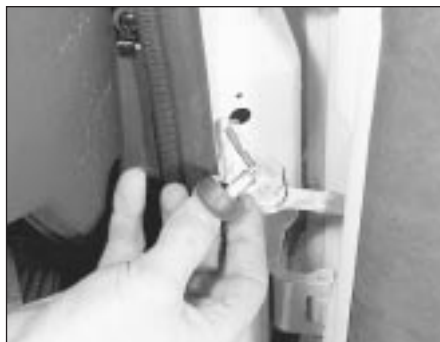
4.18 Courtesy lamp switch removal from door pillar
