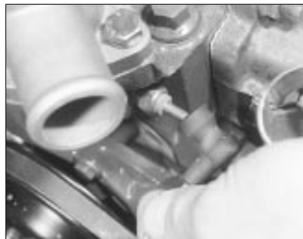
11.49b . . . and coolant temperature sender - HCS engine
