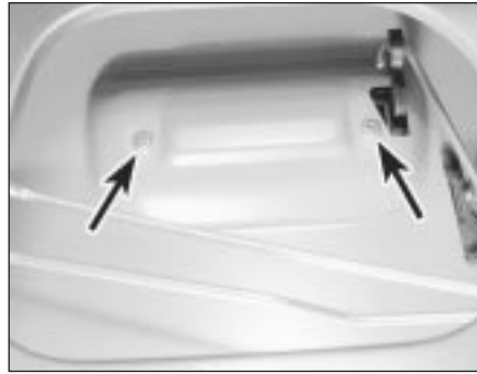
13.3 Door exterior handle retaining screws (arrowed)
