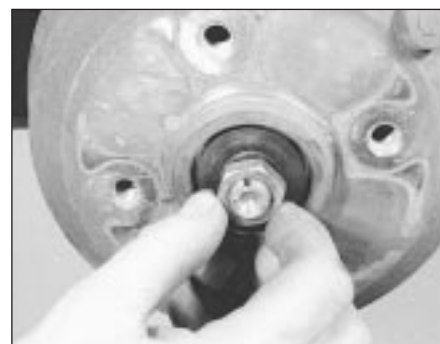
5.3c . . . then unscrew the hub nut . . .
