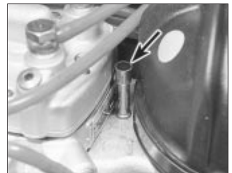
10.21 K-Jetronic system mixture adjustment screw location (arrowed)
