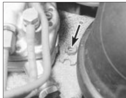
10.33 KE-Jetronic system mixture adjustment tamperproof plug (arrowed)
