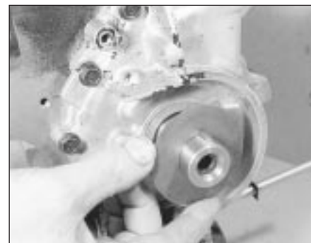
15.16 Fit the timing belt guide with its concave side towards the pump
