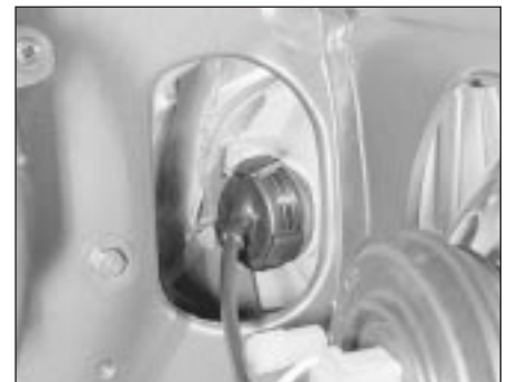
5.8 Front indicator bulbholder accessible through inner wing panel aperture
