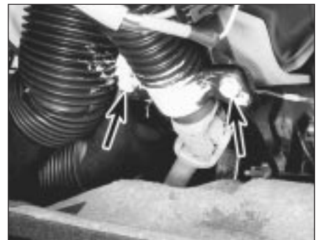
25.11a Steering column lower mounting clamp bolts (arrowed)
