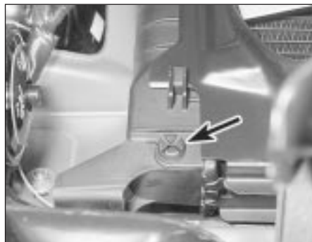
33.3 Radiator drain plug location (arrowed)
