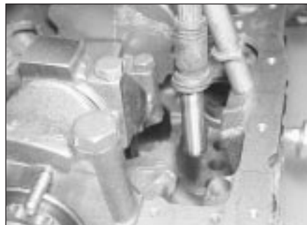
12.34 Using a valve grinding tool suction cup to withdraw the cam followers
