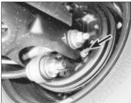
8.5 Handbrake adjustment plunger location (arrowed) on backplate
