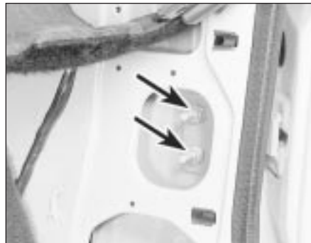
12.7a Front door lower hinge nuts (arrowed)
