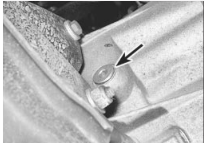
26.1b Allen type transmission filler plug (arrowed) as fitted to later models
