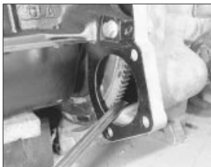
4.6 Using a stout bar to lock the flywheel ring gear
