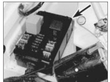
3.2b Fusebox location (arrowed) on engine compartment bulkhead - cover removed to show fuses and relays
